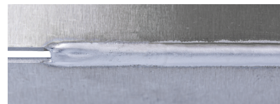
Base material: AlMg3 Filler metal: AlMg4.5 Sheet thickness: 1.5 mm Air gap: 1.5 mm
